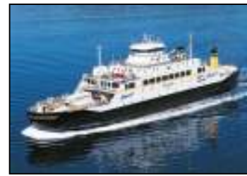
Fjord1 Gas fuelled ferry (1xC25:33L9AG retrofit)
